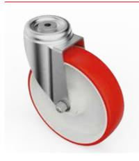
Made of a nylon 6 core and a coating of thermoplastic polyurethane, these wheels ensure a complete protection of floors and a total absence of noise while using a tread of relatively high hardness (98 Shore A)
