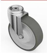
Made of a nylon 6 core and a coating of elastic injected polyurethane, these wheels ensure a complete protection of floors and a total absence of noise thanks to a tread hardness of 82 Shore A
