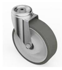
Made of a nylon 6 core and a coating of elastic injected polyurethane, these wheels ensure a complete protection of floors and a total absence of noise thanks to a tread hardness of 82 Shore A
